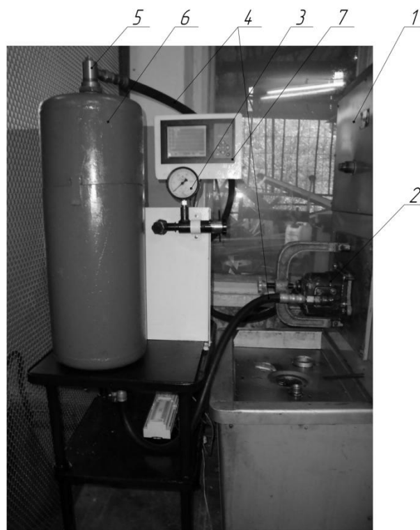
Figure – the Experimental stand for research of a hydrodynamic dispergator: 1 - stand for hydrounits testing; 2 - hydraulic pump; 3 - throttle flowmeter DR-70; 4 - hydrohoses; 5 - dispergator; 6 - hydrotank; 7 - TERMODAT 29N1 device
