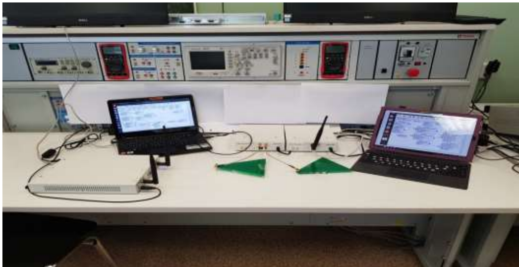
Fig.1. Configuration of Transmitter and Receiver for testing the implementation of the developed SDR transceiver in GNU Radio using real radio interface
