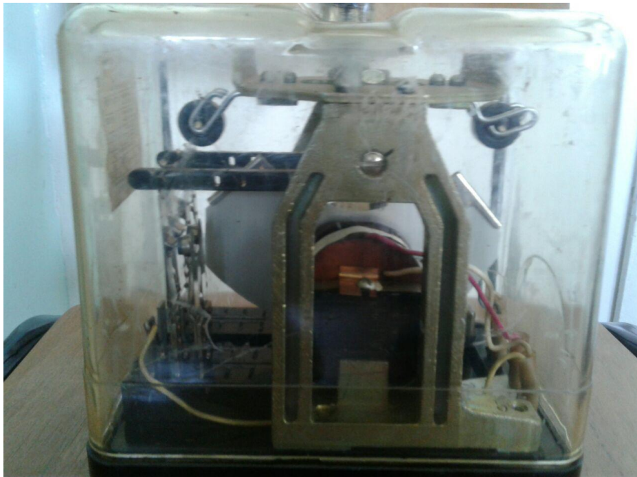
Fig 1. Relay TSP used in in the systems of railway automatics and telemechanics at railway stations
