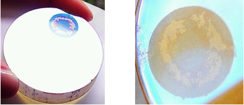
Pic. 3. To the left bottom mirror in full size. To the right enlightened area of the bottom mirror diameter of 15 mm.
